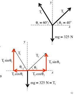
Summing forces:  $\frac{\sum F_x:}{\Rightarrow -T_1 \cos \theta_1 + T_2 \cos \theta_2 = ma_x}$   $\Rightarrow T_1 = \frac{T_2 \cos \theta_2}{\cos \theta_1}$   $= \frac{T_2 \cos 40^{\circ}}{\cos 60^{\circ}}$   $= 1.53T_2$
